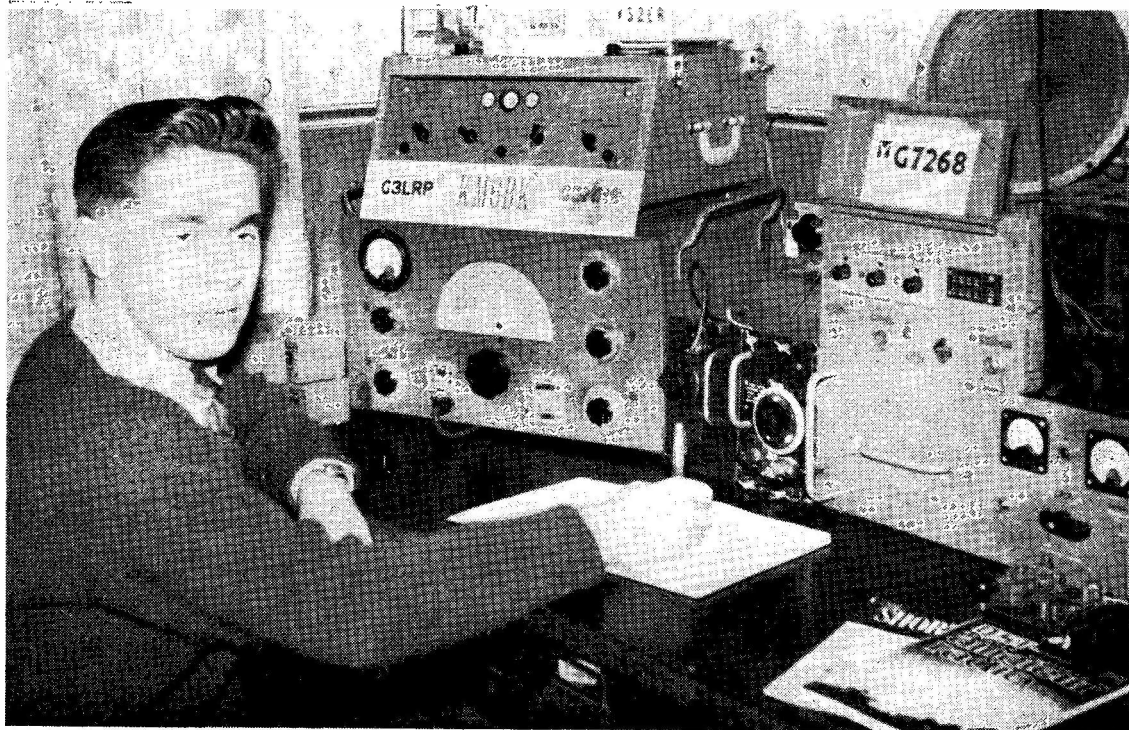
SWL Day of Sheffield is an experienced DX listener with a useful range of gear — in view are an Eddystone S.358 with RF-24 and RF-26 converters, the former for 10-15-20 metres and the latter for 6 metres; a power unit for the receiver and converter; an aerial tuning unit for all amateur bands; a Morse practice oscillator; and a tape recorder.
