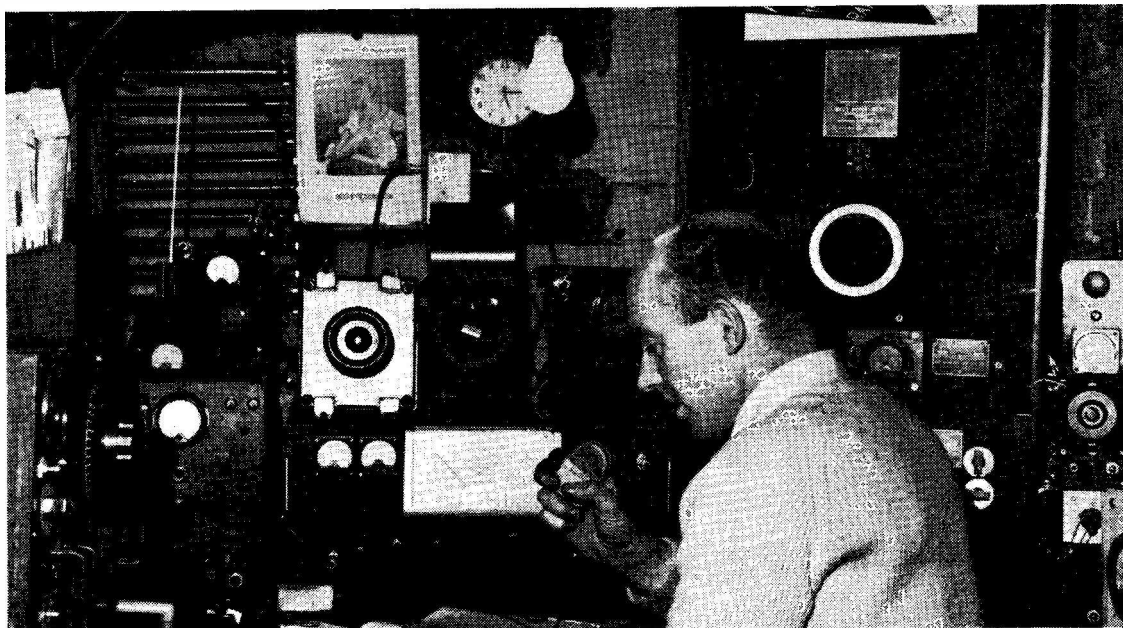
G3JHK, Stockport, Cheshire runs a home-built all-band transmitter incorporating a Geloso VFO driving a pair of 807's in parallel; these are plate-and-screen modulated by a pair of 807's in Class-B zero bias. The PA input is 140 watts, phone mainly, on 10 and 15 metres. The receiver is an HRO, and the aerial is a home-built tri-band beam, at a height of about 30 ft.
